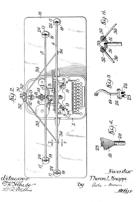
T. L. KNAPP. AUXILIABY SUPPORT FOR TYPE WRITER SHIFT FRAMES. APPLICATION FILED DEC. 27, 1907.
