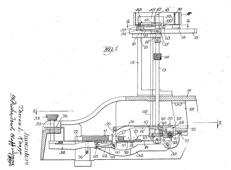
RIBBON MECHANISM FOR TYPEWRITING MACHINES
